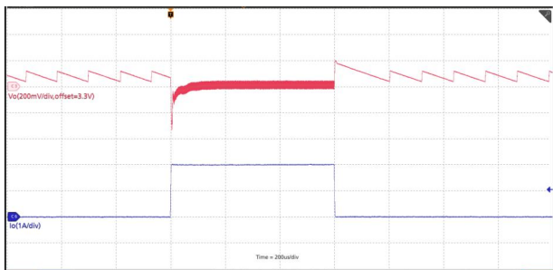
VIN=2.6V, PFM, T_A=25^{\circ}\text{C} , V_O=3.3\text{V} , I_O=10\text{mA} to 2A
